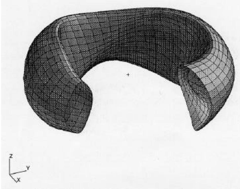
Fig. 2-4. Plasma boundary of quasi-axisymmetric configuration with  $R/a = 3.3$ .
