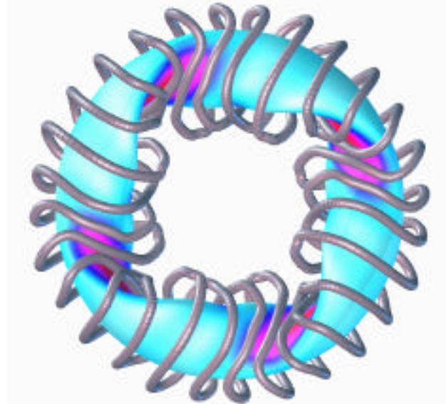
Fig. 3-4. The last closed vacuum flux surface and the coils that produce it for the four-field-period QO configuration in Figs. 3-1 and 2. Contours of constant  $|B|$  are indicated by the same color.
