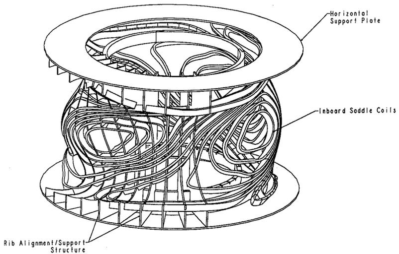
Figure 2-10 - Isometric View of Inboard Saddle Coils and In-Vessel Support Structure
