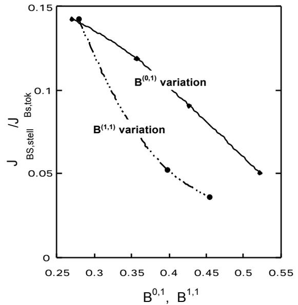
Fig. 3-3. Suppression of bootstrap current (relative to an equivalent tokamak) in 4-field-period QO devices in which the helical (1,1) or the bump y (0,1) field component of  $B$  has been increased.
