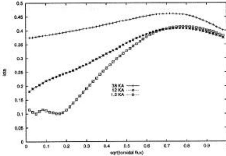
Fig. 2-5. Rotational transform profile for several values of the seed current in Configuration III.
