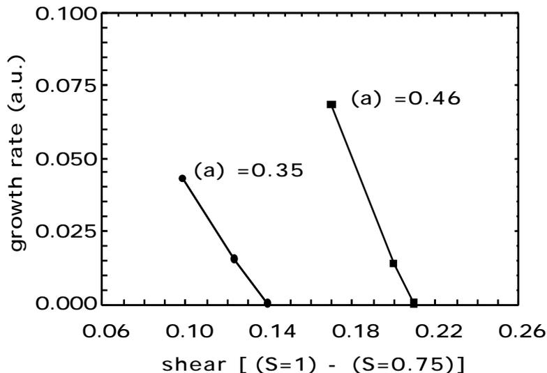
Fig. 2-7. Growth rate of the external kink mode as a function of shear at the plasma edge.
