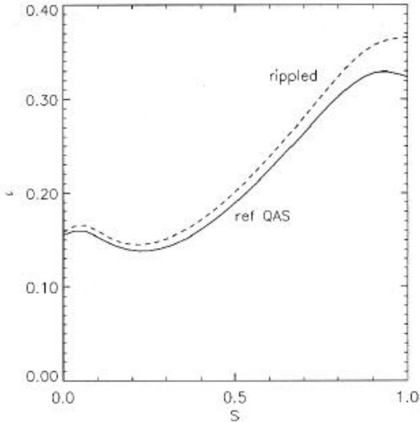
Fig. 2-8. Modification of the rotational transform profile of a quasi-axisymmetric configuration produced by a helical corrugation of the plasma boundary localized to the region near the outer midplane.
