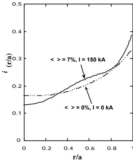
Fig. 3-2. The rotational transform profile  $i(r)$  for a four-field-period QO configuration for the vacuum configuration and for  $\langle \beta \rangle = 7\%$ . ( $R_0 = 1.5\text{-m}$  PoP case)
