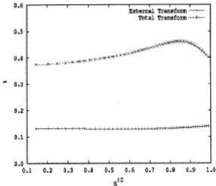
Fig. 2-3. Rotational transform profile for a three-period configuration with  $R/a = 3.3$ , flat external transform profile (Configuration III).
