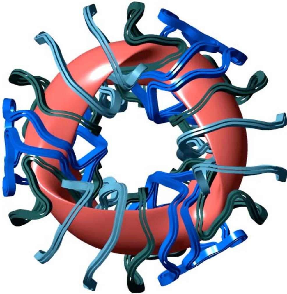
*Figure 1. NCSX plasma and modular coils.*
