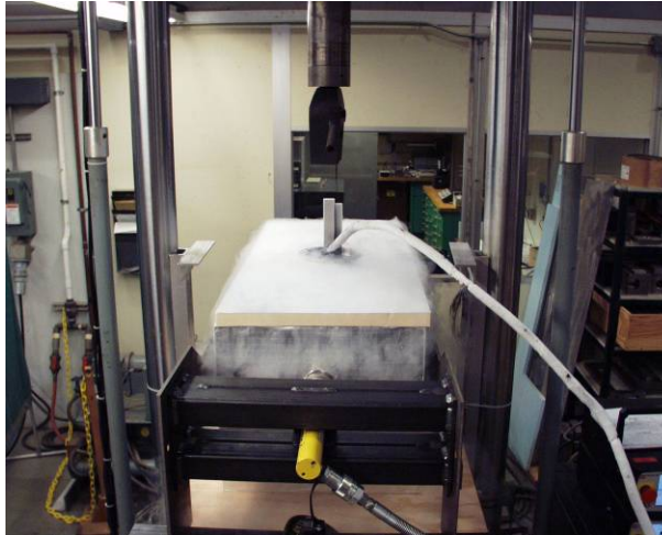
The test setup is cooled to 80 K for testing.
