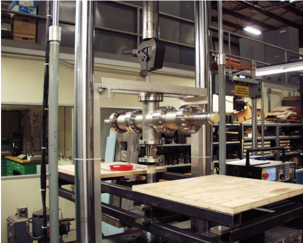
Side rams apply normal pressure to test specimens simulating bolt pressure; tensile tester applies shear load
