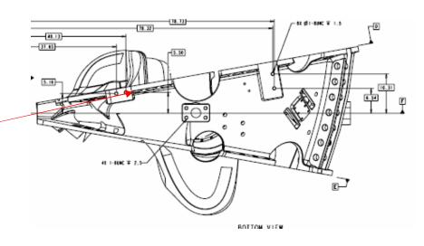
5) .400" linear on datum D outer perimeter of flange as shown above.
