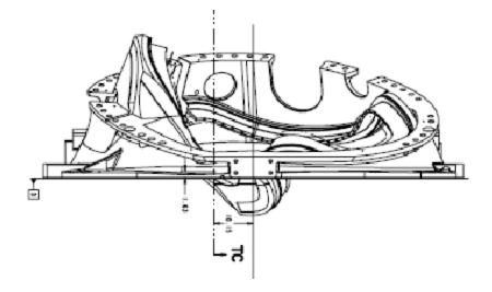
4 indications on pad between datums D and E as shown above. Although not clearly shown by picture, all indications are on this surface.
