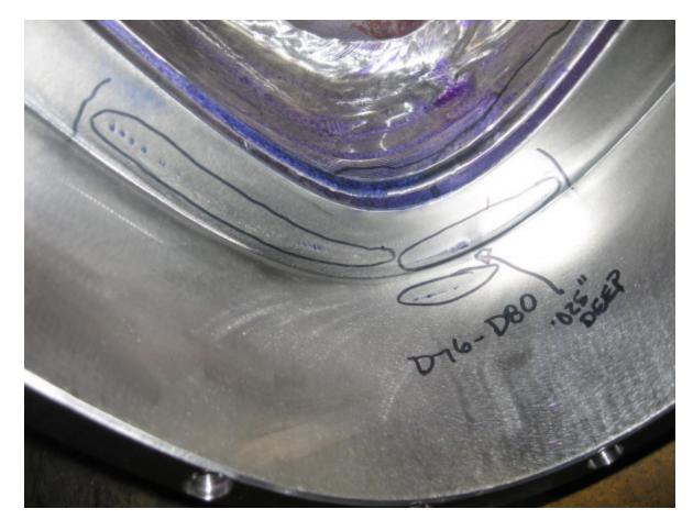
Tooling gouges between holes 76 and 80 on the datum D side of the T. Gouges are very shallow (<.005") except where noted on picture. One area measures up to .025" deep.
