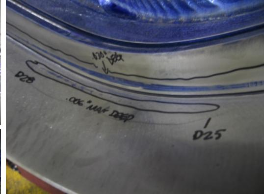
Tool gouges on long and short legs of datum D side between T holes D21 and D31 (see previous slide). Gouges are in approximately the same location as reported on B3. Long leg gouge is up to .006" deep and short leg has an area up to .03" in depth.
