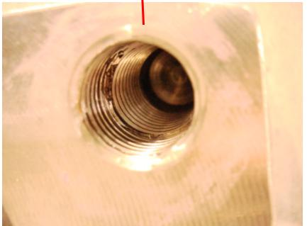
Vacuum Support Pad has damage to one of the 1"-8 tapped holes. The first .75" of the minor diameter is oversize and has damage. The hole is acceptable using a GO/NOGO thread gage.
