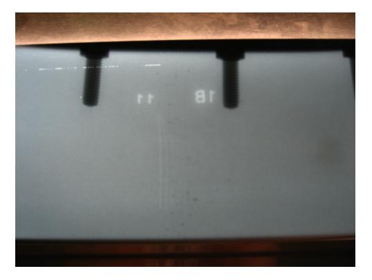
View above is of a cluster of porosity between holes 43 and 44. The largest was sized at approximately .090".
