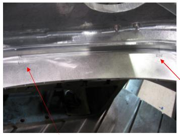
There is an undercut in the area of the 1/8" radius on both the long and short legs of E side between holes 17 and 25. The undercut extends outward in each direction approximately .300" from each wall. The undercut is deepest near E17 (approximately .040") and gradually tapers until E25.
