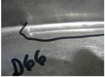
Tool gouges on D side long leg between T holes 59 and 66. Gouge near radius between D59 and D66 is <.010" in depth. Gouge at D64 is <.005" in depth.
