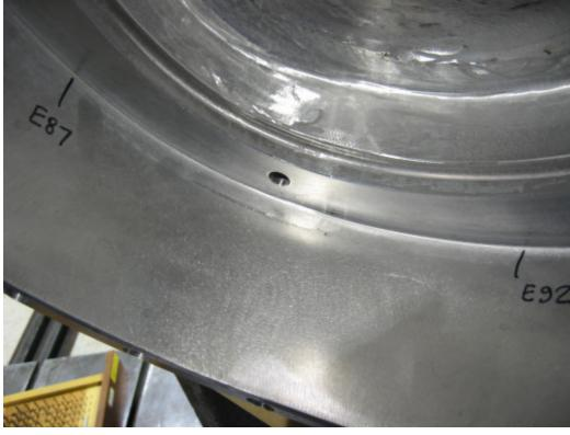
Tool gouge between holes 87 and 92 along long leg of datum E side. Depth of gouge is between .005" and .008".
