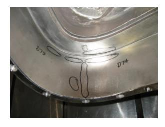
Several tool gouges on the datum D side long and short leg between T holes 74 and 79. None of these areas are greater than .010" in depth.
