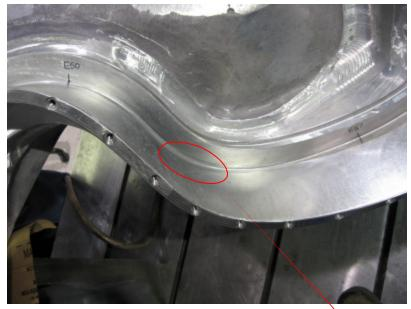
There is an undercut in the area of the 1/8" radius on both the long and short legs of E side between holes 50 and 57. The undercut extends outward in each direction approximately .200" from each wall. The undercut is deepest along the long leg between 54 and 55 (approximately .043" deep). The undercut along the short leg is less than .010" in depth.
