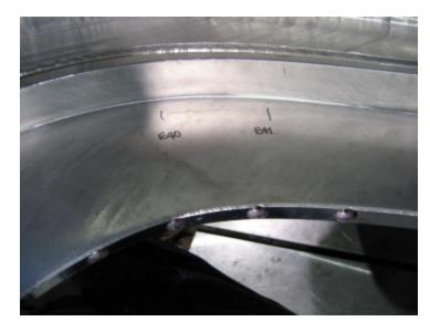
Tool gouge on E side long leg between T holes 40 and 41. This tool gouge is less than .005" deep.
