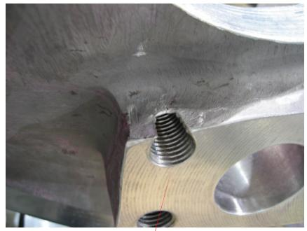
Vacuum support pad located on drawing sheet 3 zone C6 has one of the 1-8" tapped holes breaking out the side of the pad. There are approximately 5 threads breaking out the side which leaves 15 functional threads remaining.
