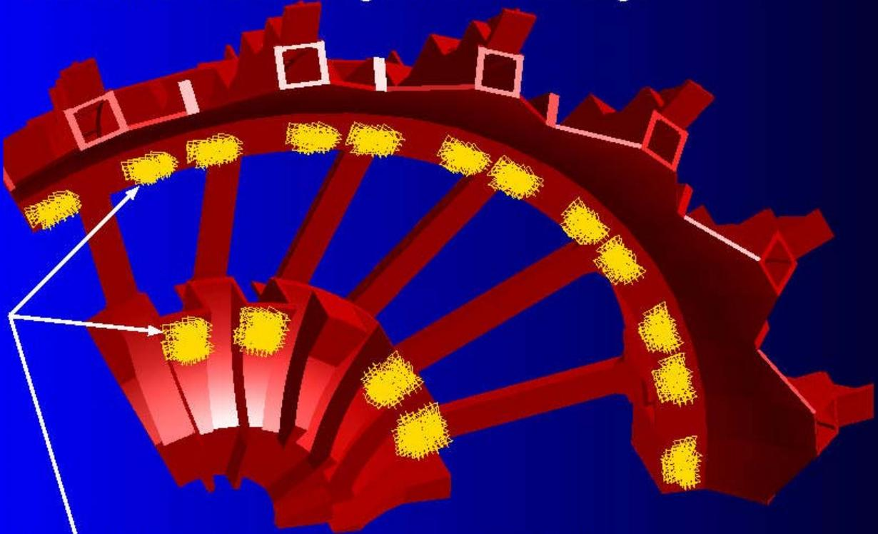
**Imposed R & Z Displacements =  $(r \text{ or } z)(CTE)(dT)$**
