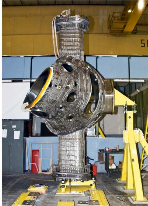
Figure 5 - A Vacuum Vessel Sub-Assembly
