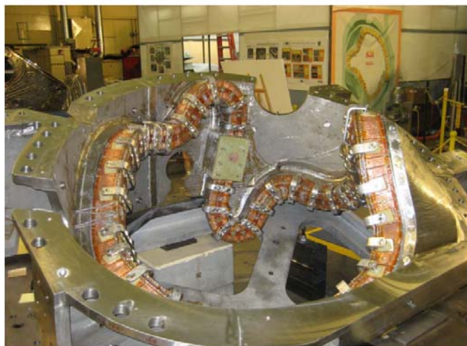
Figure 1 - A Type C Modular Coil after Vacuum Impregnation and Installation of Coil Clamps
