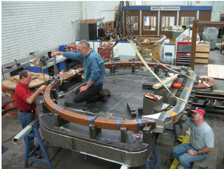
Figure 4 - Quality control tests being performed on a NCSX TF coil at the Manufacturer
