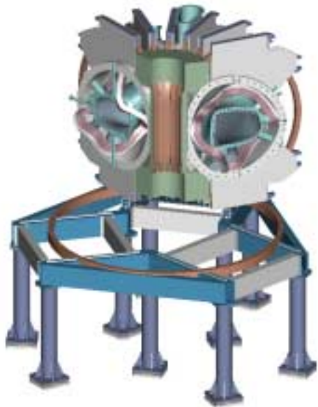
Field period lowered onto machine base in position ~ 500 mm radially outward
