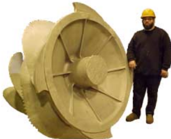
Pulper Rotor Alloy: Grade 318 (Modified CF8M) Casting Weight: Appx 6,500 lb. Size: 6 ft. Dia, 8 ft. High
