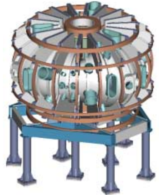
Field periods connected after radial motion, PF coils raised/lowered into position
