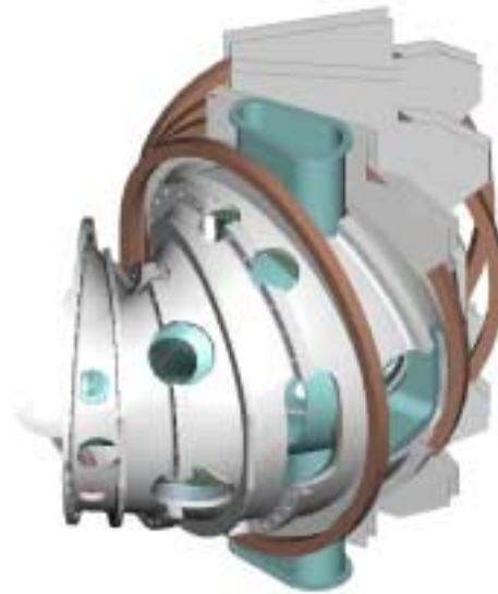
Add TF coils and out-of-plane support structure
