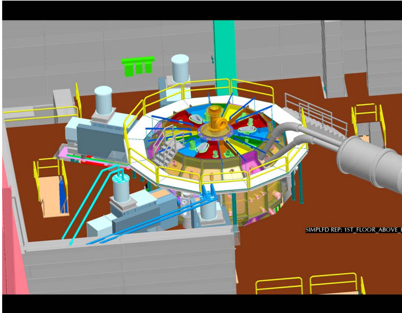
Integration of cryostat with current vintage facilities in the NCSX Test Cell (looking South)
