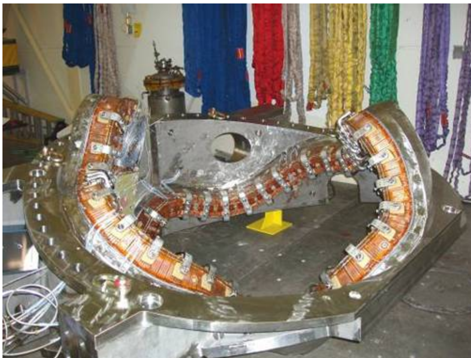
Figure 14: Modular coil with clamps installed.
