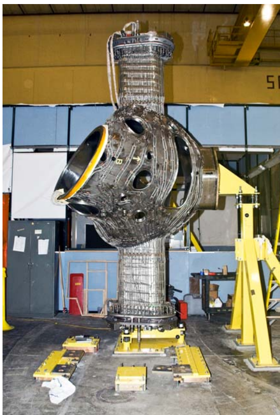
Figure 5: Vacuum vessel sub-assembly with cooling hoses and diagnostic instrumentation installed.
