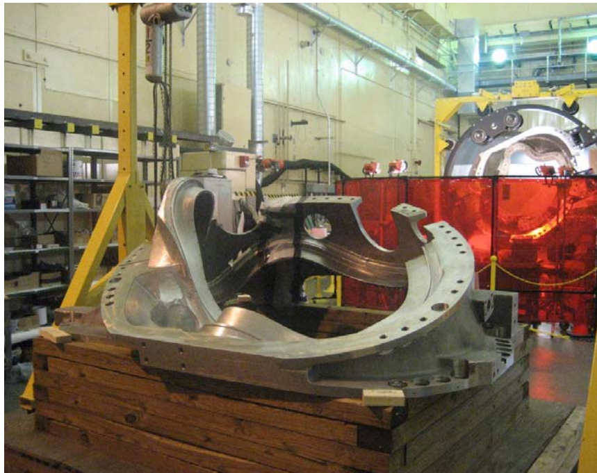
Figure 11: Modular coil winding form fabricated by industry and delivered to PPPL.
