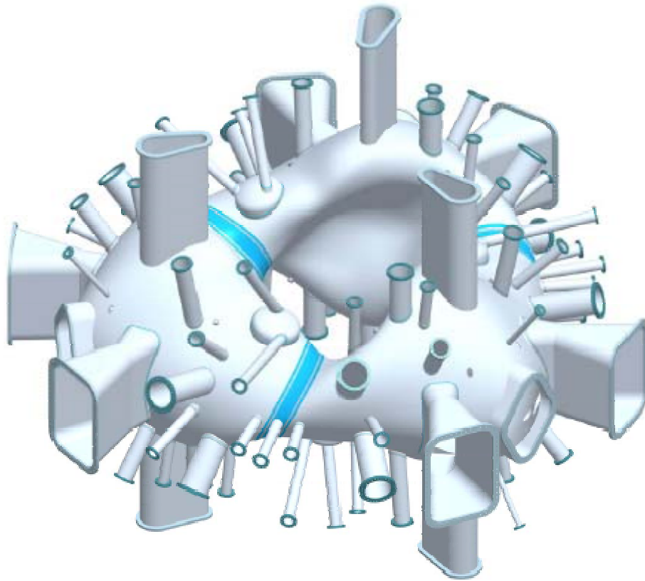
Figure 3: NCSX vacuum vessel design.
