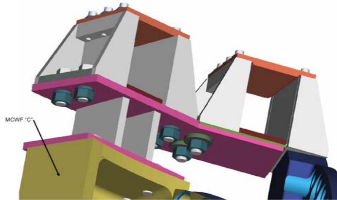
TF Inner Supports "B" to "C" Span
