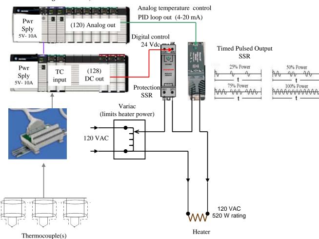
ControlLogix Processor, 1756 I/O
