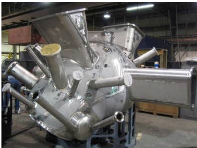
Figure 4: One of three NCSX vacuum vessel sectors fabricated by industry and delivered to PPPL. (The port extensions were later temporarily removed during assembly operations.)
