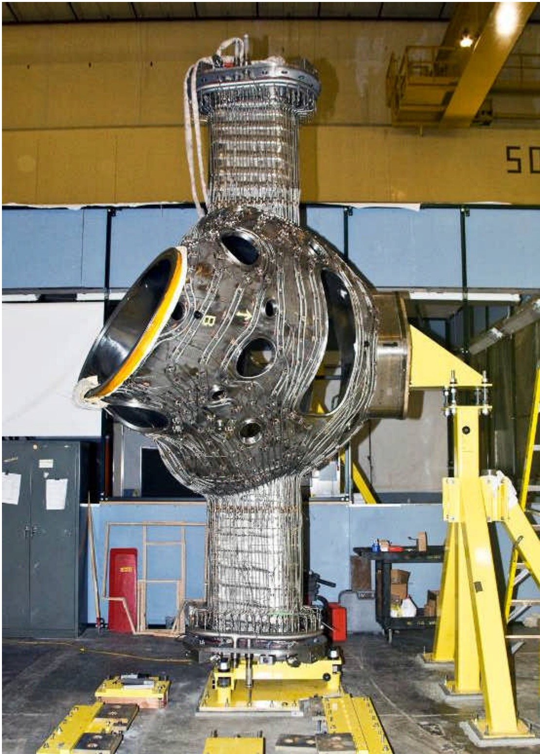
Figure 5: Vacuum vessel sub-assembly with cooling hoses and diagnostic instrumentation installed.
