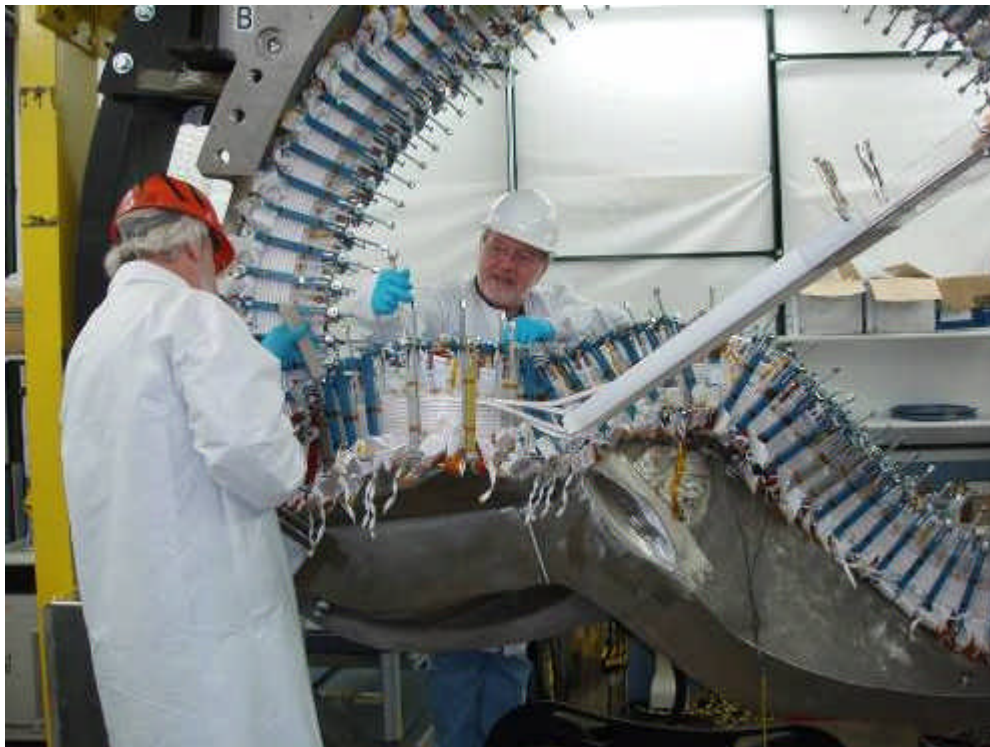
Figure 15: Modular coil winding operations at PPPL.
