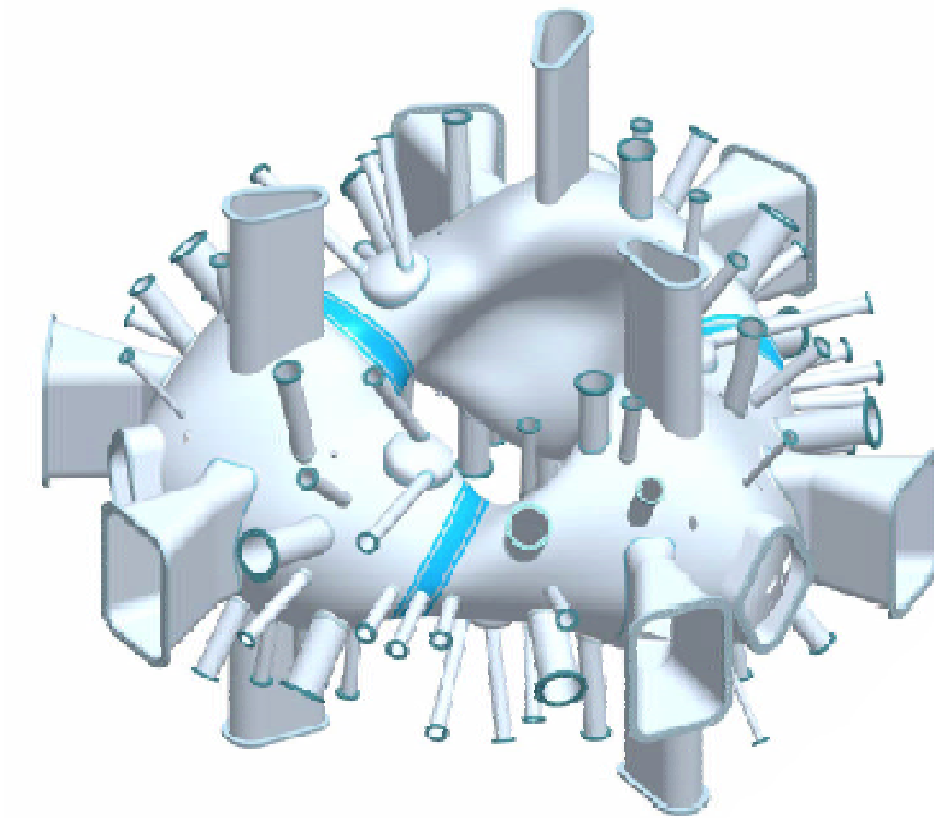
Figure 3: NCSX vacuum vessel design.
