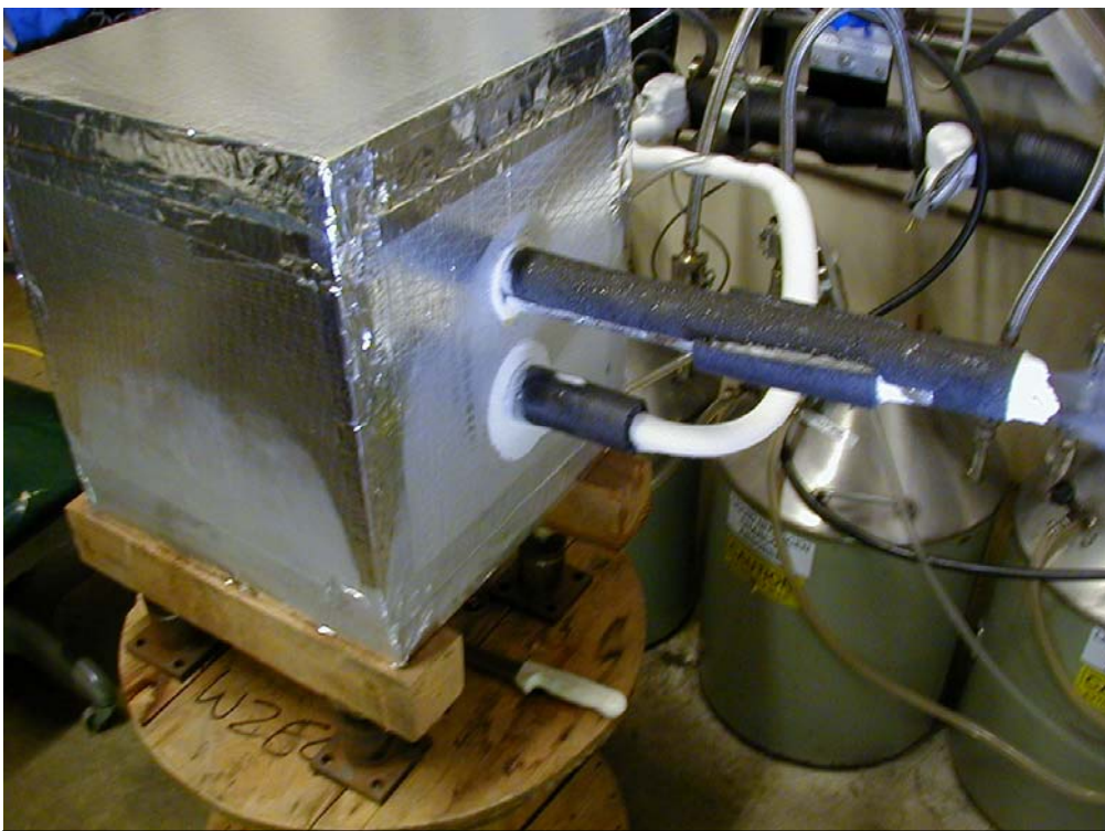
Figure 6 Cryostat/Insulation Test Module
