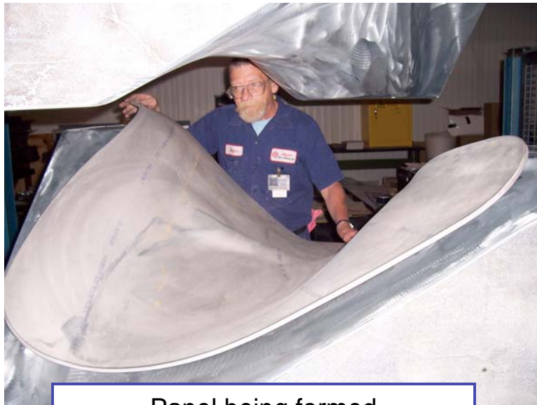
Panel being formed
