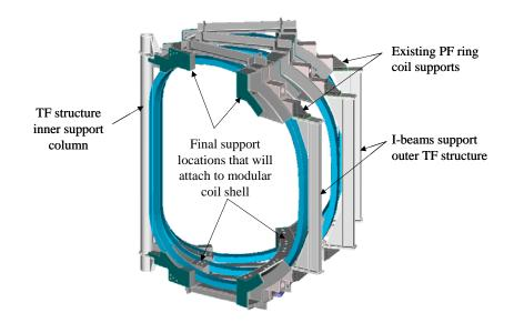
The baseline plan for final assembly is to set (all?) the TF coils back  $\sim 1/4$ " so that they do not wedge prior to the modular coils in one field period contacting the mating coils in the adjacent field period. (A gap between mating coil structures would seem to be needed as well.)
