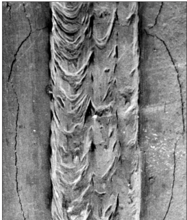
Figure 20. Failure in INCONEL alloy X-750 induced by residual welding stress at a 2-in. (51-mm) thick joint which was welded in the age-hardened condition and re-aged at 1300°F (705°C) for 20 h after welding.
