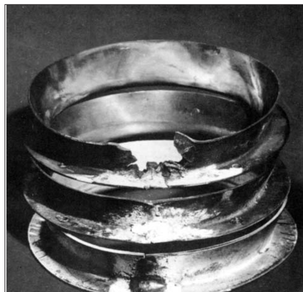
Figure 25. Attack by molten welding flux.
