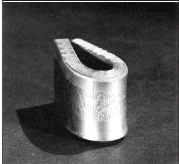
Figure 27. Longitudinal bend-test specimen in which weld runs central and parallel to the long edge.
