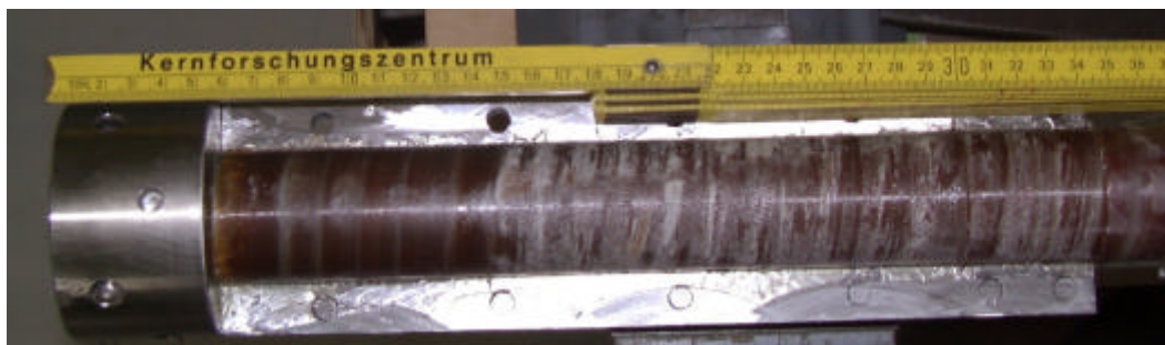
Figure 24. Photograph of the structure after the test. The half of the clamp has been removed.
