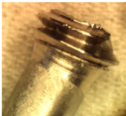
Figure 73. Failure position of the specimen and the etched weld zone.
