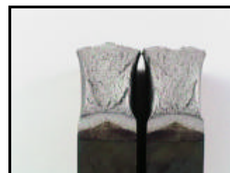
Figure 38. Obtained crack profile after loading of specimen #2 at 4.2 K. Large crack tunneling
