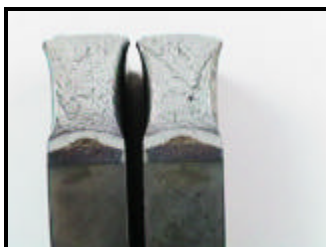
Figure 37. Obtained crack profile after loading of specimen #1 at 4.2 K. Large crack tunneling
