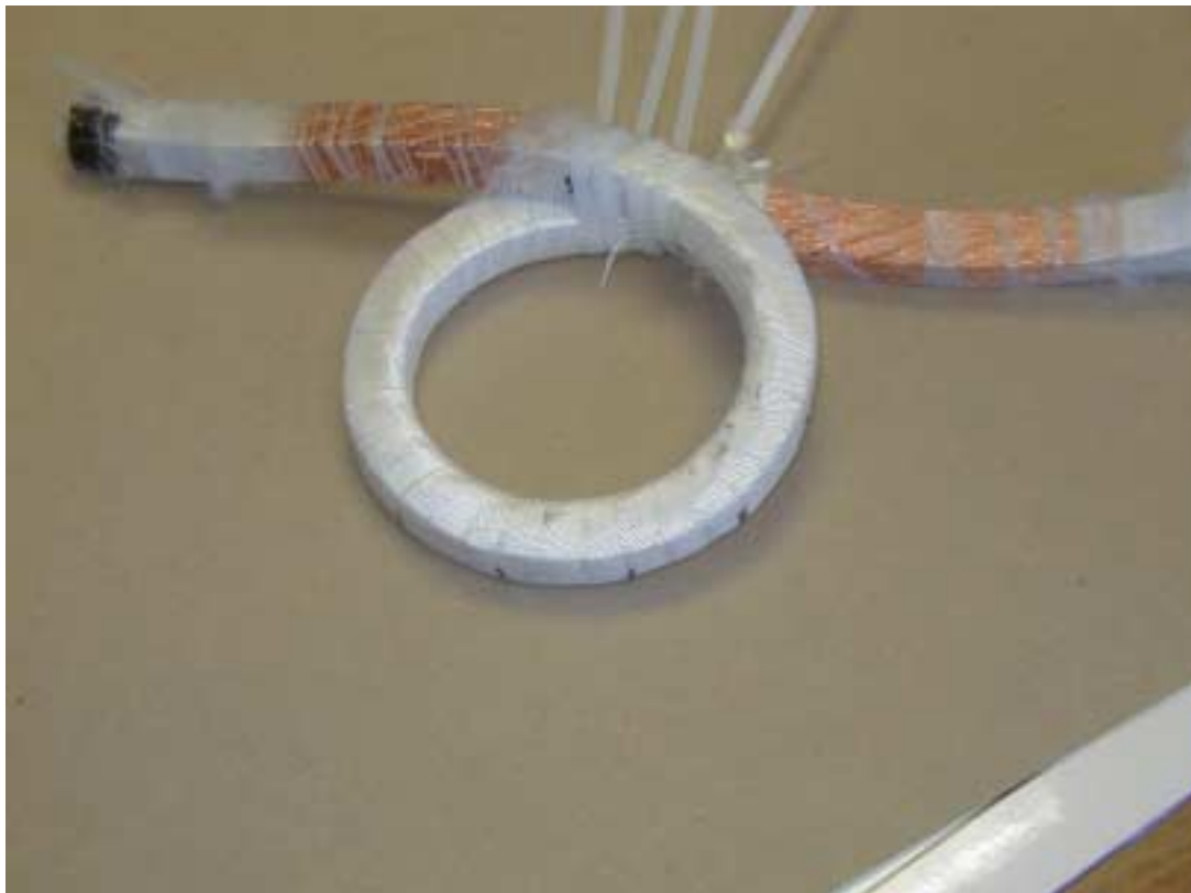
Figure 1- Trial #1 “Conductor Removed from Mandrel”
