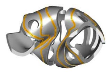
Two sets of double pancake windings with space in between for coolant septum and locating structure.
