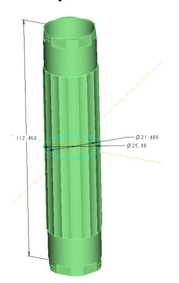
Segmented bucking cylinder keyed for torsional continuity
