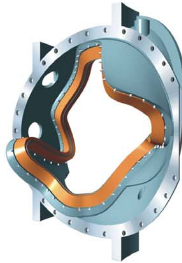
Conductor wound directly into structure
