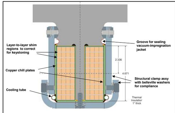
**Figure 3 - Modular coil details**
