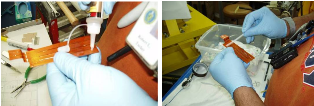
Figure 27-Applying Adhesive to Vertical Cladding
