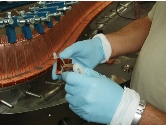
Figure 30- Applying Adhesive to Horizontal Cladding
