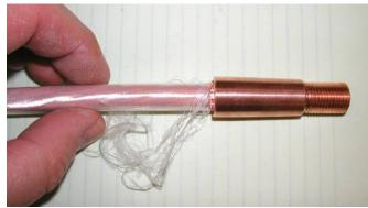
**Figure 15- Conductor in Connector**
