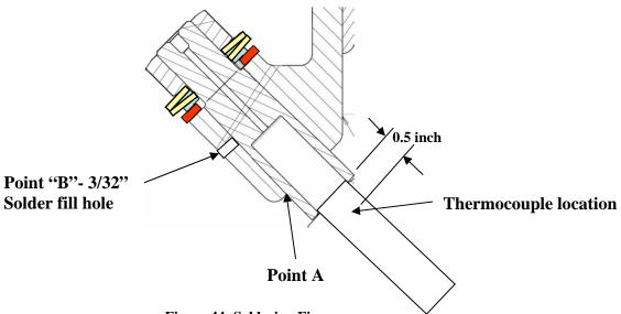
**Figure 44- Soldering Figure**
