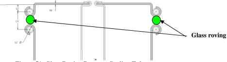
Figure 51- Glass Roving Between Cooling Tubes
