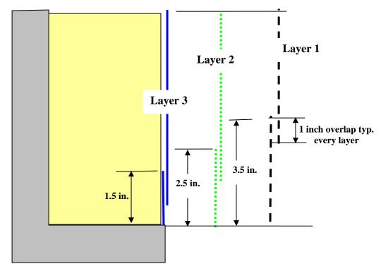
Figure 26- Groundwrap Overlap Scheme
