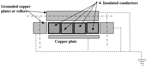
Figure 23-Schematic of Turn Insulation Tester
