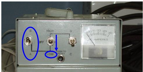
Figure 42- Front Face "Nibco" Soldering Unit
