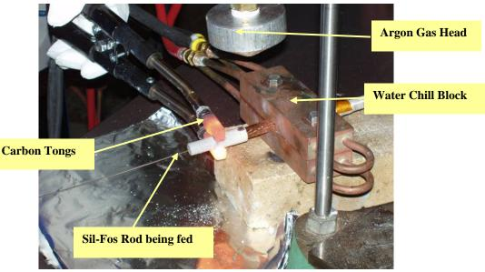
**Figure 16- Basic Setup for Brazing Lead Connectors**
