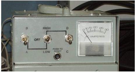
Figure 30- Front Face- "Nibco Soldering Unit Control
