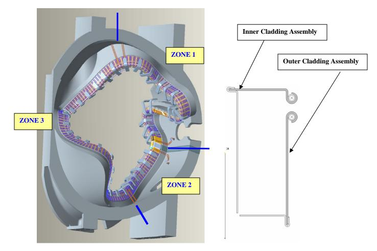
Figure 35- Cooling Tube Zone Identification
