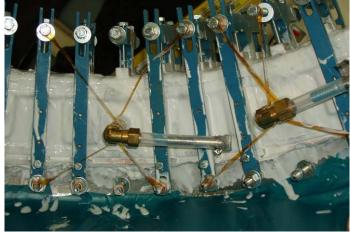
Figure 55- Bag Mold with Painted RTV 11
