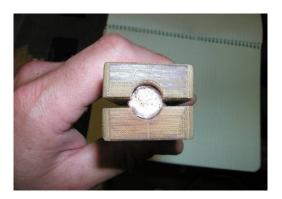
**Figure 13-Conductor in Forming Block**
