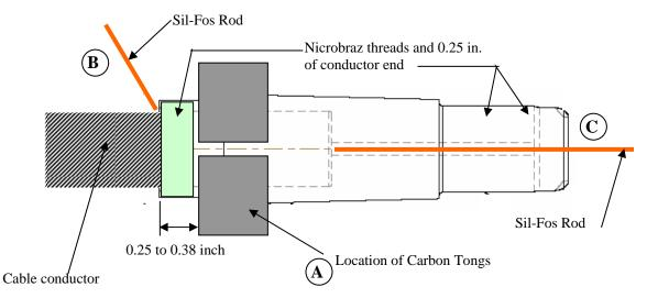
Figure 18- Carbon Tong Positioning & Sil-Fos Feed
