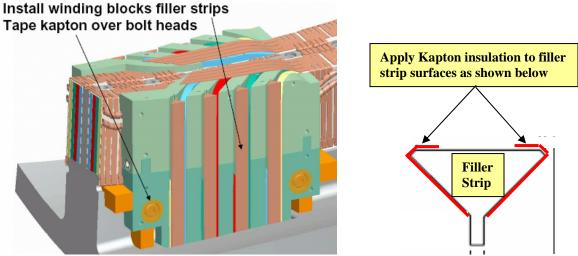
**Figure 46- Winding Block Filler Strips**
