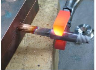
Figure 19- Heating Copper Connector
