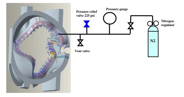
**Figure 36- Pressure Test Schematic**
