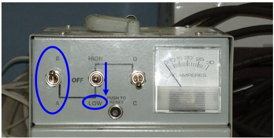
Figure 17- Front Face- "Nibco" Braze Unit Control
