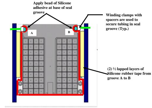
**Figure 52- Installation of Bag Mold**
