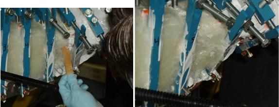
Figure 57-Application Epoxy Glass Shell
