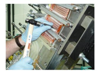
**Figure 27- Staking Chill Plates**
