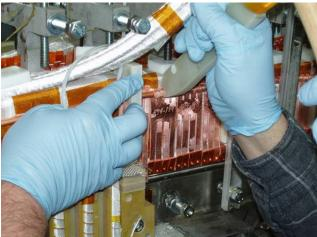
**Figure 29- Setting Chill Plate and Tubing**
