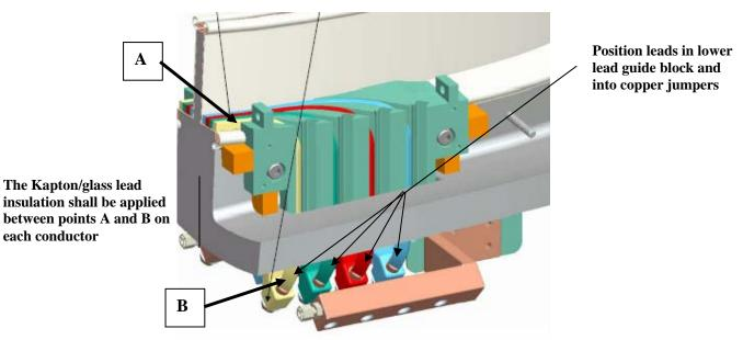
Figure 22- Positioning leads
