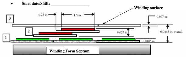
Figure 6- Groundwrap scheme
