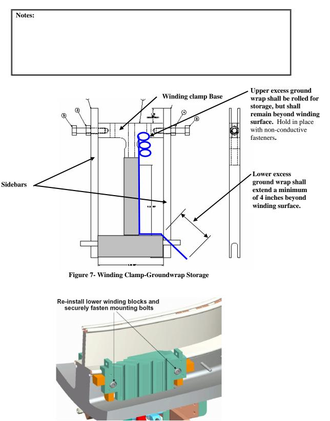
Figure 8- Re-installation of Lower Winding Blocks
