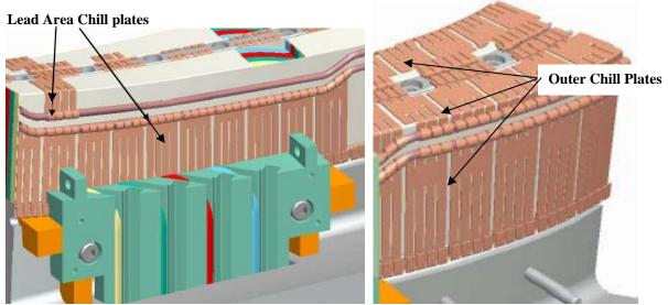
Figure 33- Chill Plates in Lead Area
