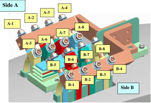
**Figure 41- Final Terminal Connections Identification**
