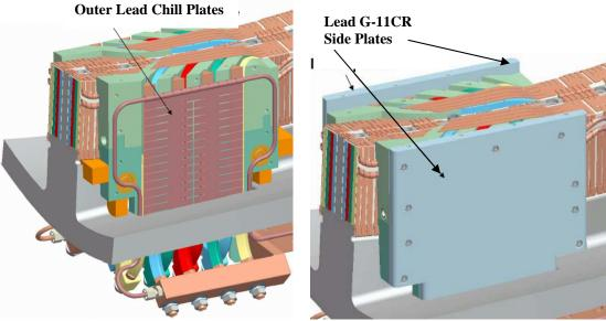
Figure 47- Outer Lead Area Chill Plate
