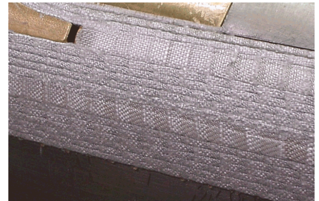
CTD-1012PX ceramic pre-preg as applied on FNAL half-coil
