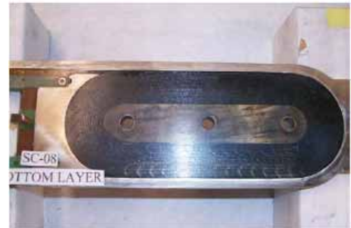
LBNL sub-scale coil fabricated using CTD ceramic insulation and CTD-101 VPI resin
