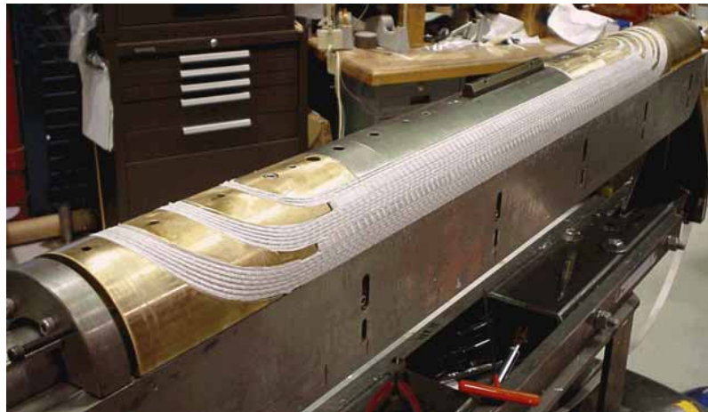
FNAL half-coil fabricated using CTD-1012Px insulation system
