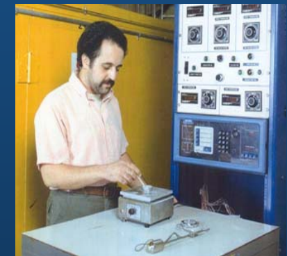
"Scrambled Egg" test to verify Gel temperature
