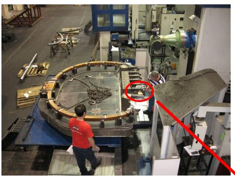
A precisely machined wedge template is used to inspect the wedge angle as well as the location of coil with respect to the intersecting axis formed by the angle
