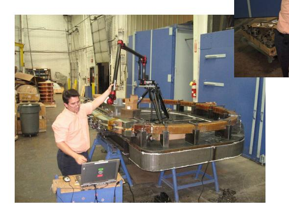
PPPL verified Everson tooling and measurement techniques on TF Coil#1 on location at Everson
