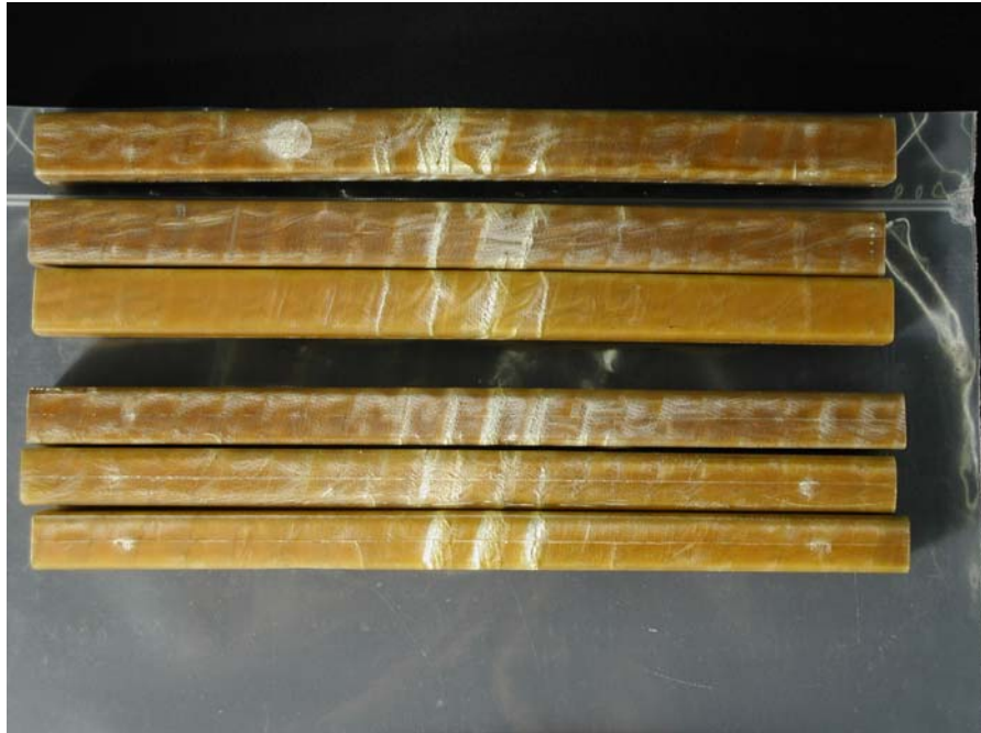
Figure 1. Failure mode for Flexure specimens at 295 K (flatwise direction at top, edgewise direction at bottom).
