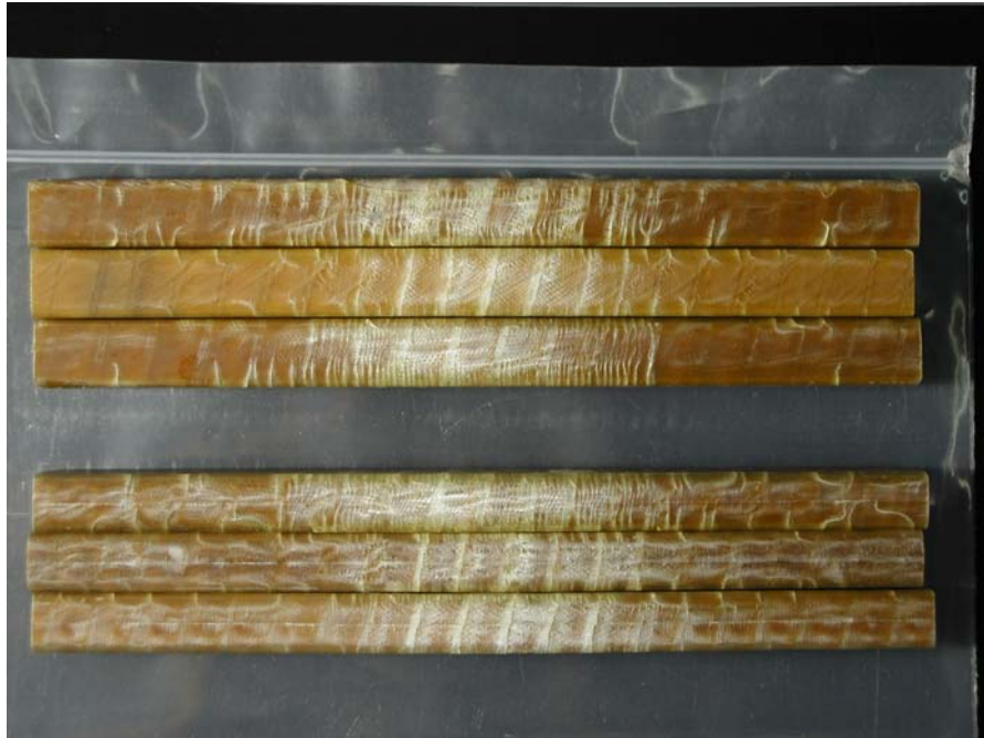
Figure 3. Failure mode for Flexure specimens at 100 K (flatwise direction at top, edgewise direction at bottom).
