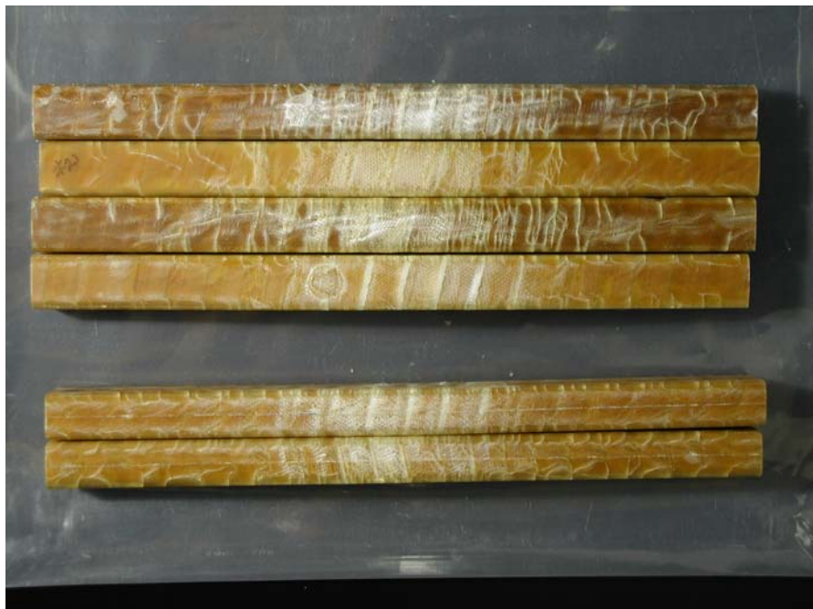
Figure 4. Failure mode for Flexure specimens at 76 K (flatwise direction at top, edgewise direction at bottom).
