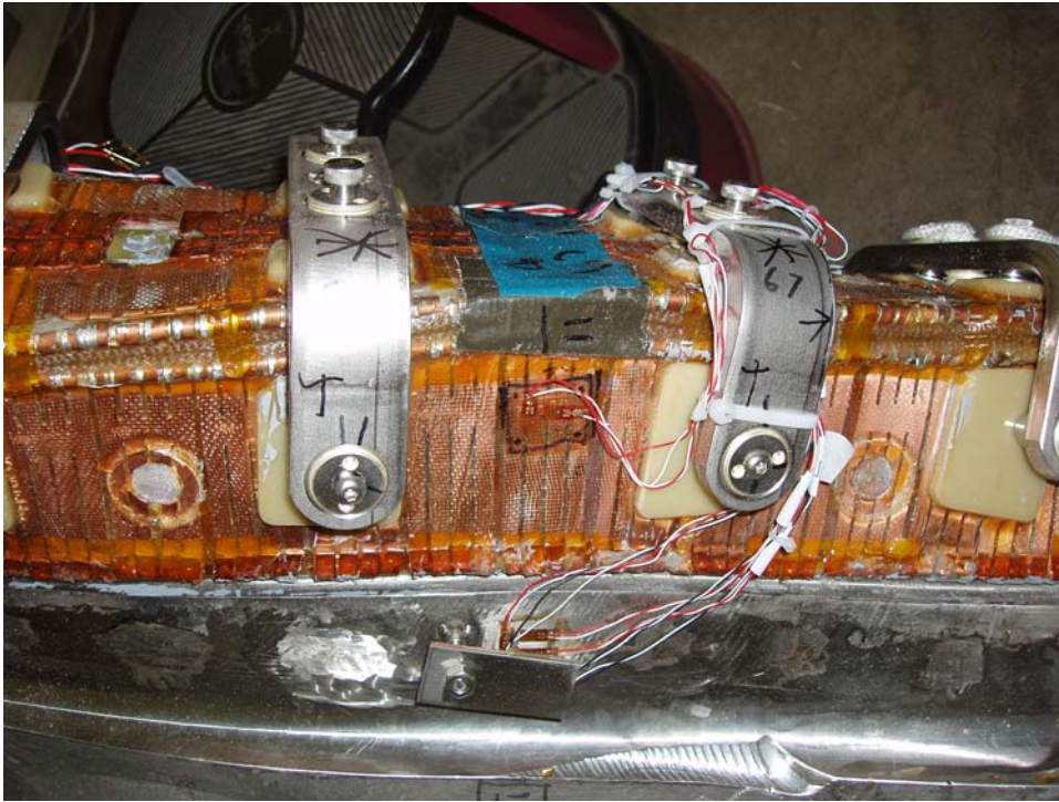
Figure 5-34 Strain gages at Clamp 68 - Side B
