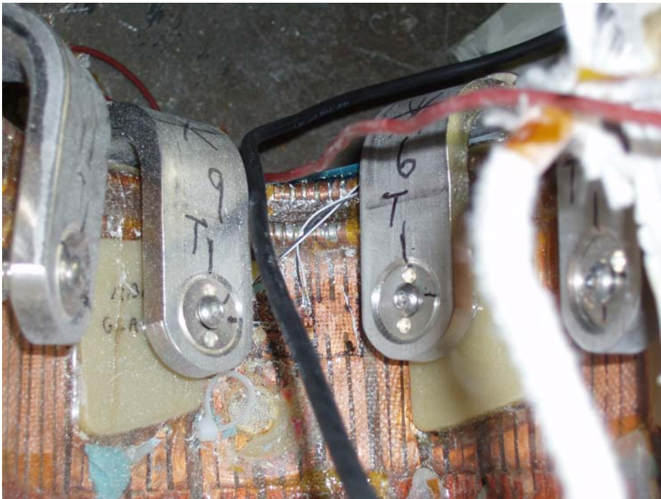
Figure 5-39 Winding pack strain gage (dummy) at Clamp 7 - Side B
