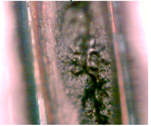
Photo 4: Weld Sample 1- Incomplete fusion on the backside
