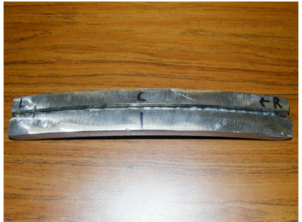
Photo 10: Weld Sample 7- Backside complete fusion
