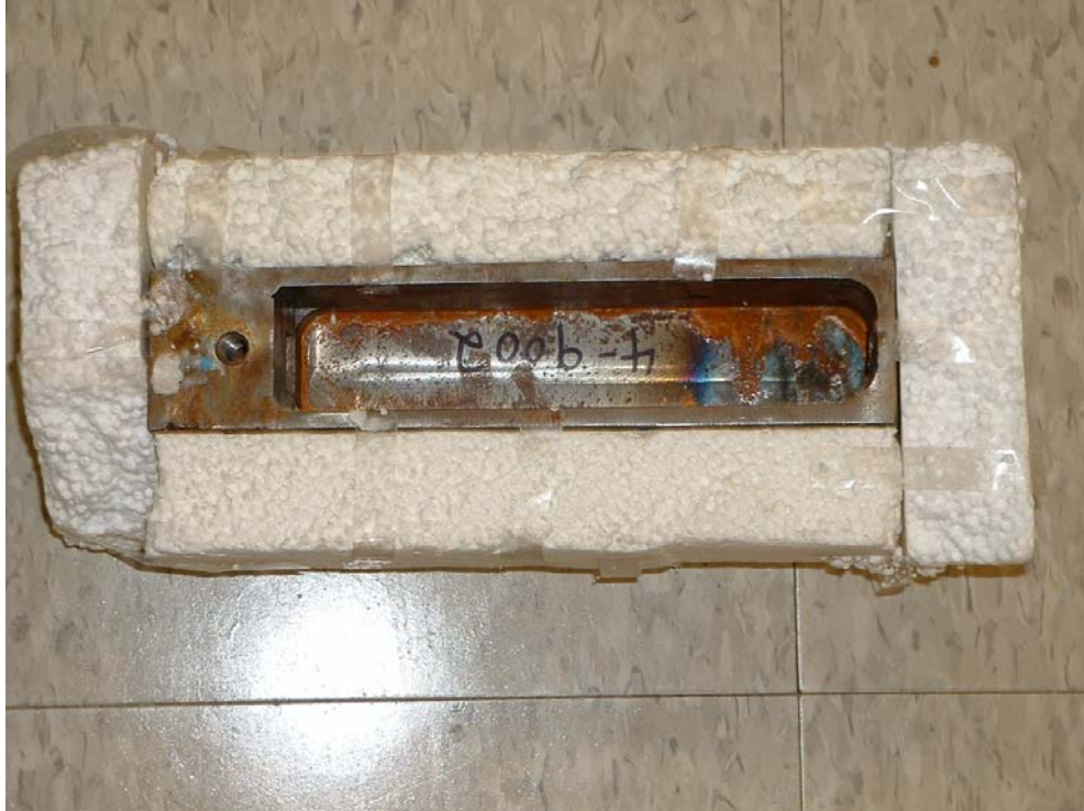
Figure 4. Top view of the photograph of the cantilever beam bending fixture (without a specimen). The fixture is insulated by means surrounding it with a 1-inch thick Styrofoam.
