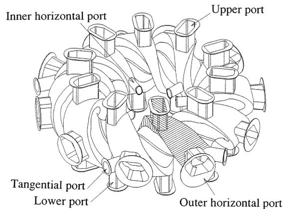
Fig. 1. Plasma vacuum vessel with five types of ports.
