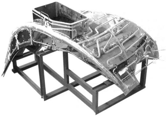
Fig. 6. Half sector unit of torus shape and side plates for helical coil space. The surface is covered by a 80 K shield plate and pipes for helium gas.
