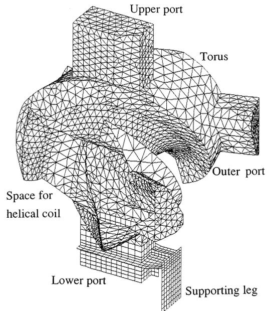
Fig. 2. The analytical model of the LHD plasma vacuum vessel with ports and supporting leg.
