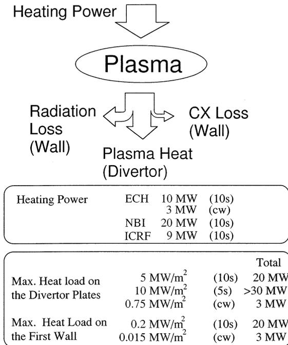
Fig. 3. Heat loads on the plasma vacuum vessel.
