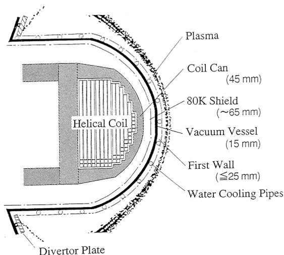
Fig. 4. Radial build between helical coil and vacuum vessel.
