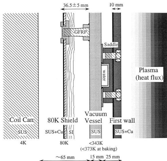
Fig. 5. Components between the coil can and the plasma in the radial build.
