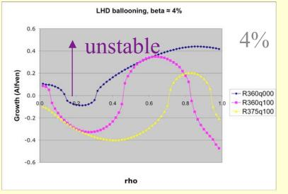
COBRA code (R. Sanchez) Ballooning *only* Very fast (seconds)  $p \propto (1-\rho^2)$  (imposed) Mostly stable at lower  $\beta$ At higher  $\beta$ , unstable regions depend on configuration
