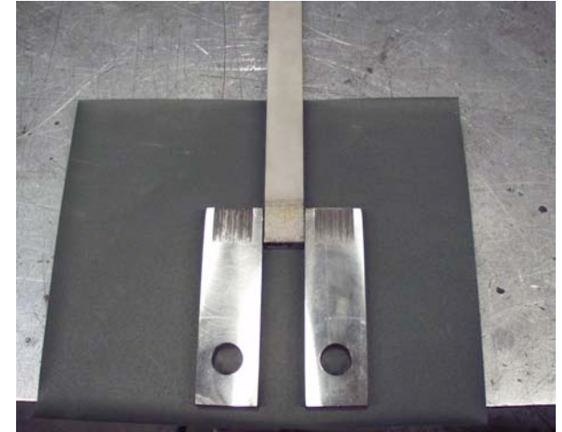
Test specimen – two alumina coated SS sideplates sandwich SS center bar.
