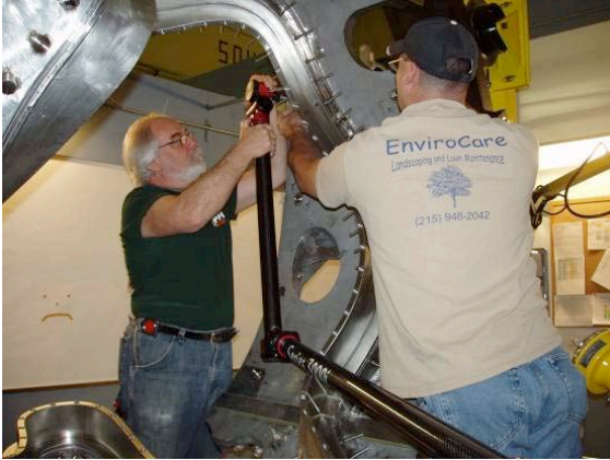
These figures show surface measurements being taken using the “Romer” arm
