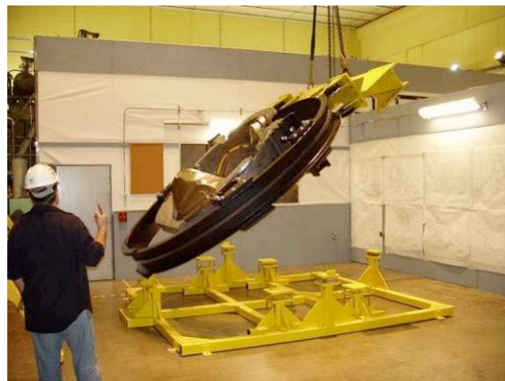
Transferring Coil to Vertical Position for Transport
