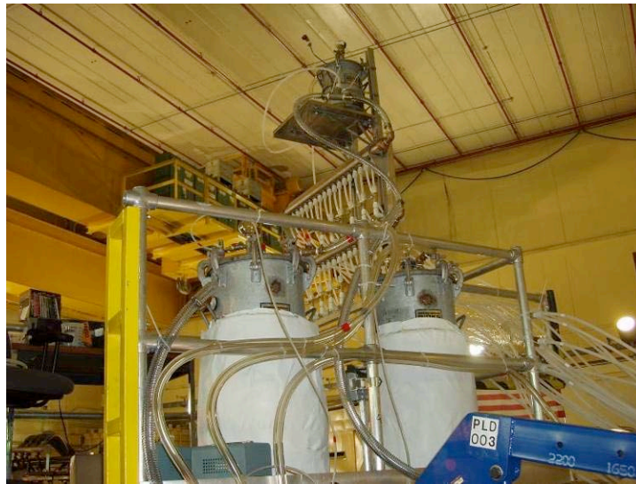
Epoxy Delivery Control Station
