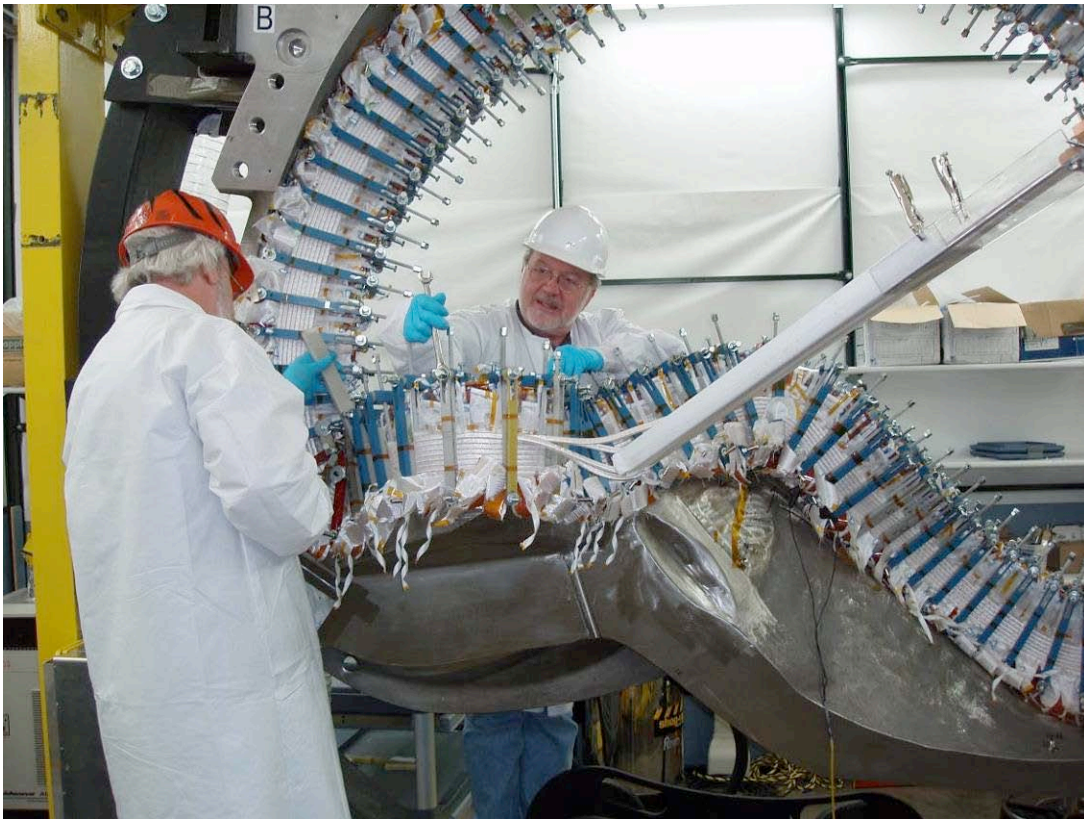
Modular Coil Winding Operation
