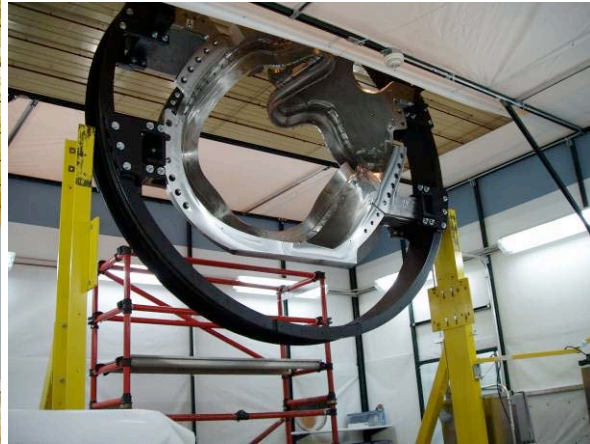
Transferring Coil Assembly to Winding Station
