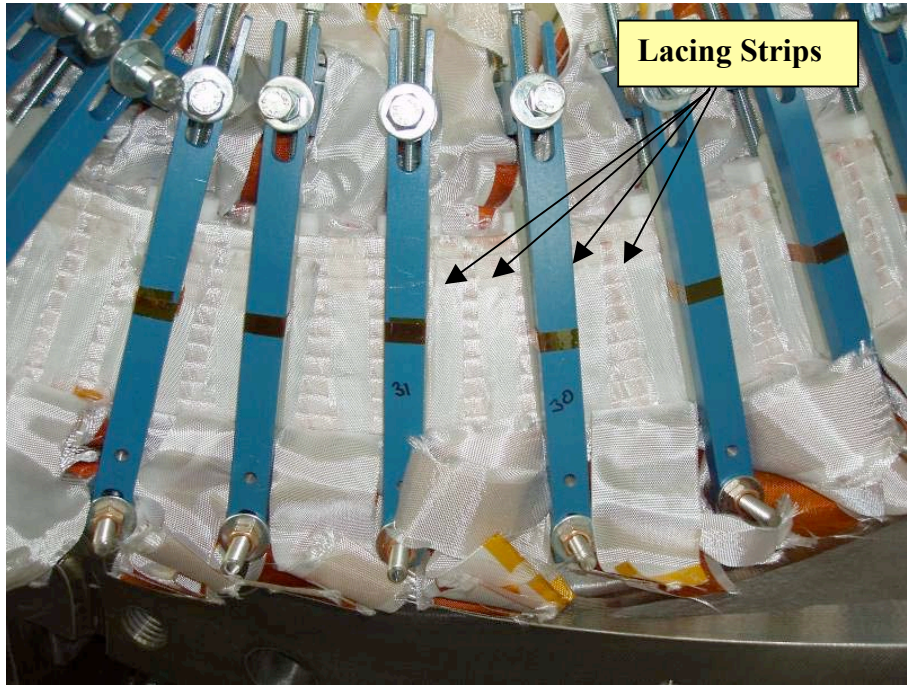
Glass Tape Lacing Strips Secured
