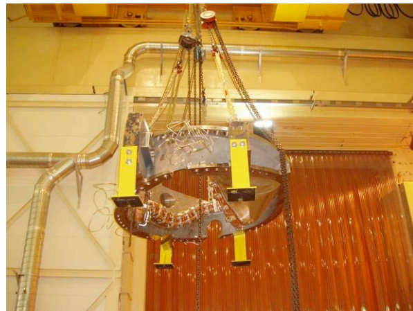
Coil Being Removed from Ring Assembly
