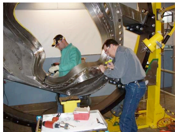
Quality Control Representative is measuring the Magnetic Permeability Using a Severn Gauge
