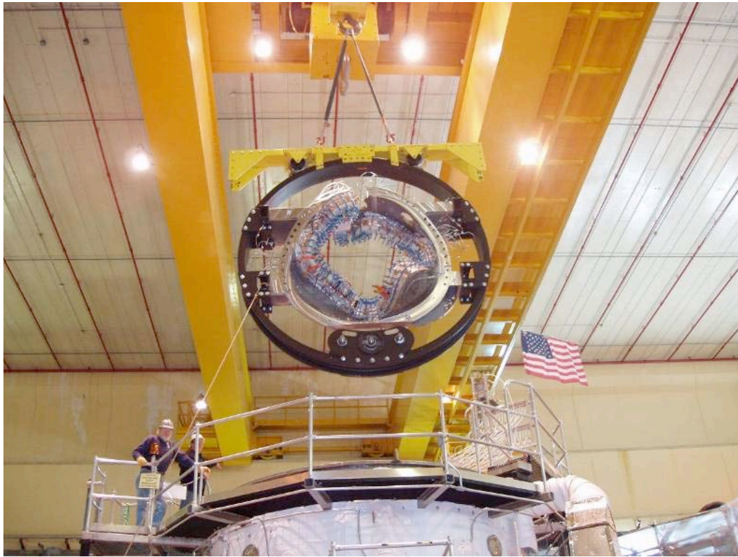
Modular Coil being lifted into the Autoclave
