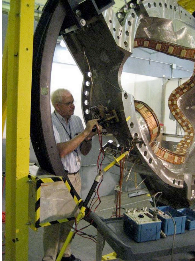
Measuring the Coil Resistance
