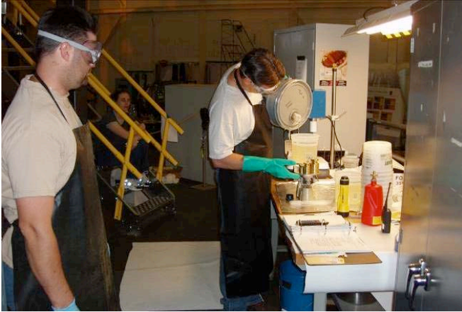
Epoxy Being Weighed prior to VPI
