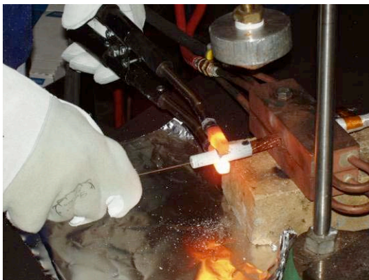
Brazing Copper Lugs onto Conductor
