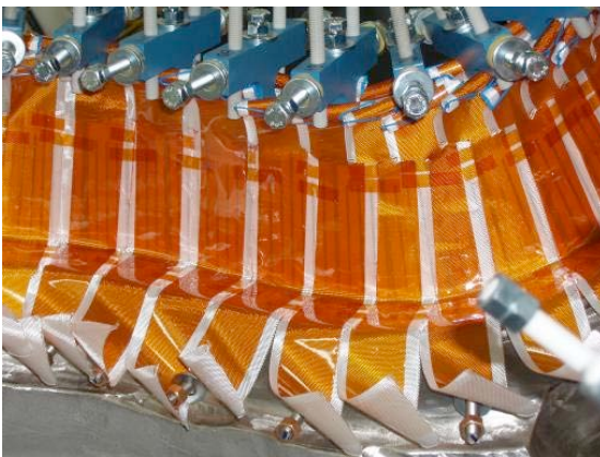
Applying Ground wrap insulation
