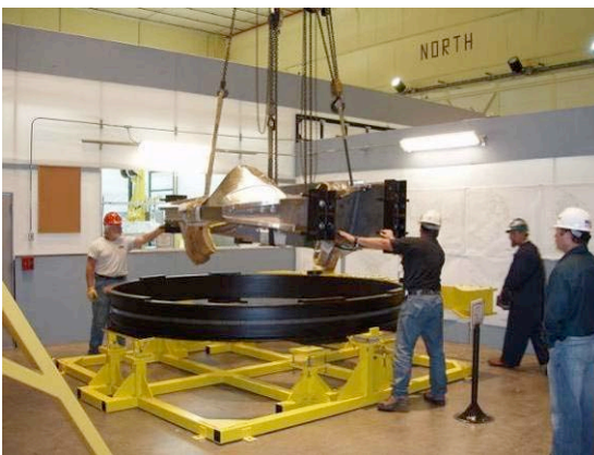
Loading Winding Form Into Support Ring
