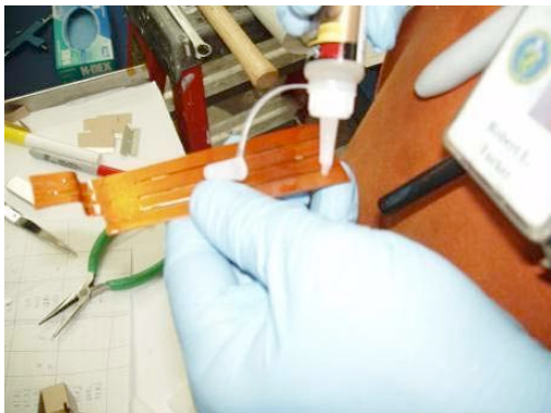
Application of 3M Adhesive to Kapton
