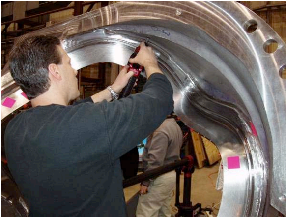
Using “Romer” Mechanical Measurement arm to verify surfaces
