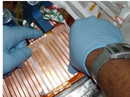
Application of 3M Adhesive to Kapton
