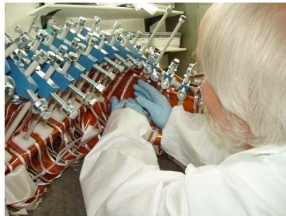
Applying Ground wrap insulation
