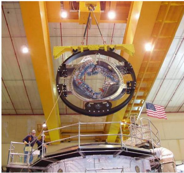
Figure 10- Installation of Modular Coil into Autoclave
