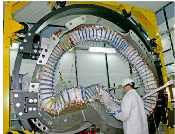
Figure 5- Coil Winding Operation
