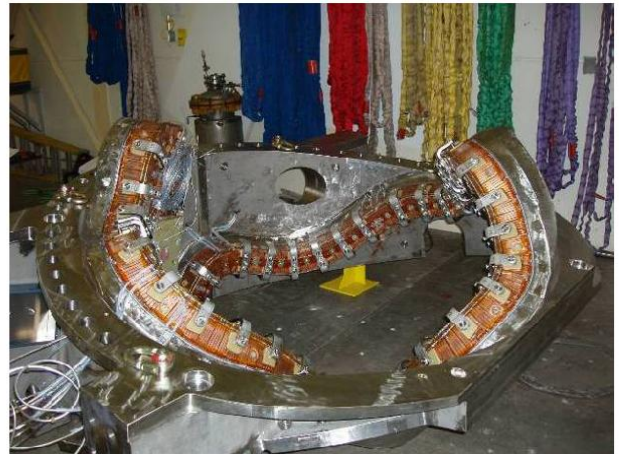
Figure 11- Finished Modular Coil
