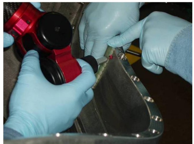
Figure 2- Measuring Winding Surface using CMM "Romer" and Template
