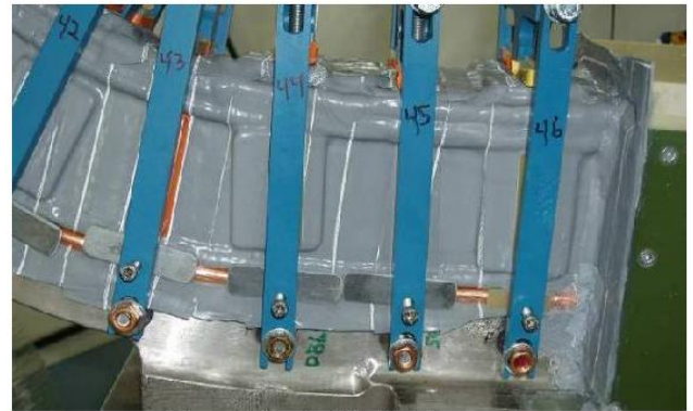
Figure 8- Bag Mold under Vacuum
