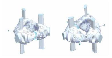
Figure 2. NCSX VACUUM VESSEL Distribution of Flux Loops
