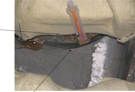
Note the recess milled into B coil. This will keep the bag from moving around.
