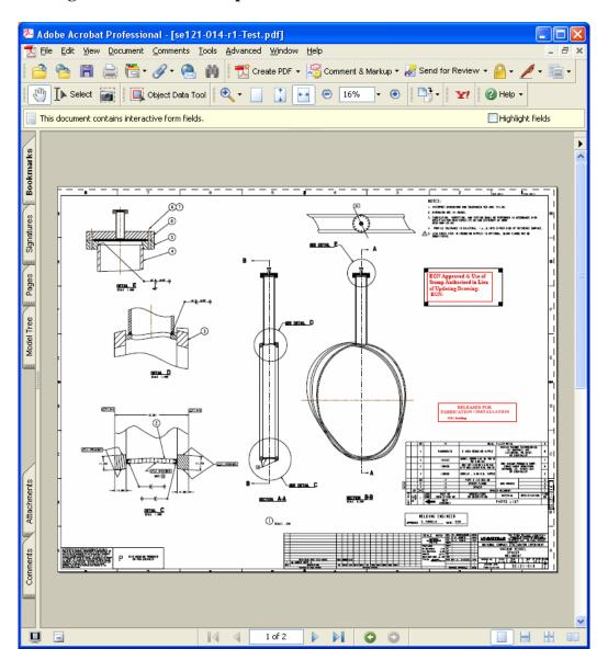
• Place the necessary text (e.g., ECN Number, and drawing Rev and stamp revision number/letter) by selecting: Tools => Advanced Editing => Text Field Tool and place text block where desired at size desired. Next select "Hand Tool" and click within the text field block and type the information desired – note that size of text is usually set to Auto to maximize readability.
