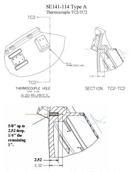
We are requesting a change to the thermocouple in section TC2-TC2 of drawing SE141-114 sheet 9 similar to what has already been approved on the thermocouple at location TC1-TC1.
