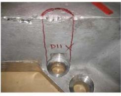
In order to expedite the rework of B1 and B2, MTM is requesting the option to bore the counterbore relief completely through the area in red (from the top of the support leg to the counterbore). The cut would extend into the leg approximately 1.3" over a distance of 8.5" to the counterbore face. This applies to hole 11 in the D flange only.
