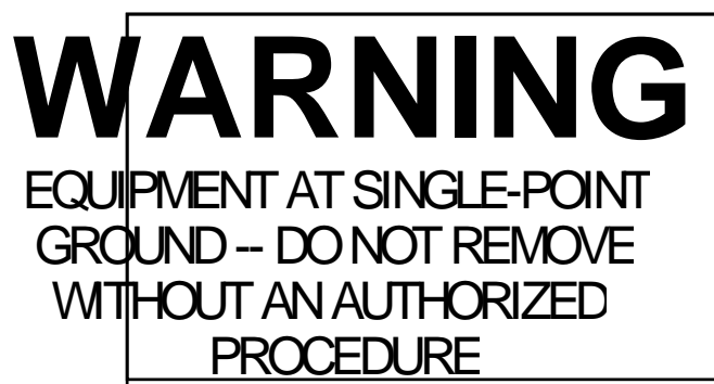
Figure 9.6-1 Single Point Ground Warning Label
